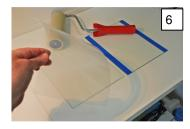
Treat the upper glass plate with 2% Dichlorodimethylsilane (Repel Silane) in a <u>fume-hood</u>. (Solution prevents adhesion of gels to glass) (**Pic 4**) (Bring 2 ml Silane in 98 ml Petrolether 40-60°C). Store in refrigerator.
